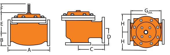
For maximum efficiency, the OCV control valve should be mounted in a piping system so that the valve bonnet (cover) is in the top position. Other positions are acceptable but may not allow the valve to function to its fullest and safest potential. In particular, please consult the factory before installing 8" and larger valves, or any valves with a limit switch, in positions other than described. Space should be taken into consideration when mounting valves and their pilot systems.
