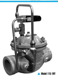
The Model 115-1NY is used in a water supply line in conjunction with fire sprinkler piping. Its basic purpose is to divert the potable water usage to the fire sprinkler line.
