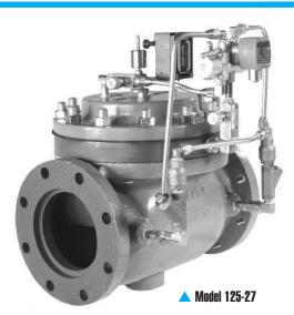
The Model 125-27, primarily designed for use with centrifugal booster pumps, can also be used on well pumps with relatively shallow lifts where the pump design permits starting against a closed valve.
