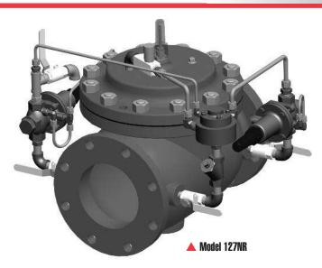
The Model 127NR is used in conjunction with a smaller, parallel valve in those systems that must provide both normal usage and fire flow. The small valve provides normal flow at a lower outlet pressure. The 127NR provides fire flow at a higher outlet pressure.
