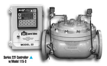
The Model 22F Electronic Flow Control Valve provides user flow control with extreme stability over a wide range of flow. Combining the advantages of simplicity and line pressure operation with the features of electronic control, the valve is able to interface with SCADA systems to provide remote control and programmable variable logic. The electronic feature allows for a wider range of operation, simplifying valve
