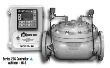
The Model 22S Electronic Pressure Sustaining/Back Pressure Valve provides user pressure control with extreme stability over a wide range of flow. Combining the advantages of simplicity and line pressure operation with the features of electronic control, the valve is able to interface with SCADA systems to provide remote control and programmable variable logic. The electronic feature allows for a wider range of operation, simplifying valve sizing.
