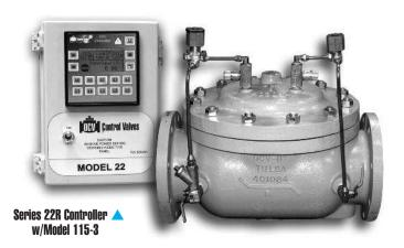
The Model 22R Electronic Pressure Reducing Valve provides user pressure control with extreme stability over a wide range of flow. Combining the advantages of simplicity and line pressure operation with the features of electronic control, the valve is able to interface with SCADA systems to provide remote control and programmable variable logic. The electronic feature allows for a wider range of operation, simplifying valve
