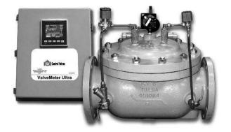
The 22VMU is a self-contained, electronic flow measuring and flow control system. Based upon the variables of valve differential pressure and valve position, the ValveMeter Ultra automatically calculates, displays and controls the flow to the control set point. With the ValveMeter Ultra, there is no need for a separate flow meter in the line.
