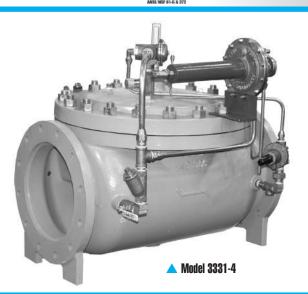
The Model 3331-4 is applicable anywhere it is necessary to automatically maintain the water level in elevated storage tanks or reservoirs, and where it is desired to allow the tank level to fall a given amount before refilling to allow greater turnover and/or to prevent stagnation. Such applications occur in:
