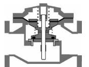
The upper spool assembly drops. The valve is now ready for normal forward flow operation.
