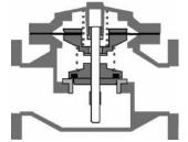
Valve inlet pressure is less than valve outlet pressure. The lift check (lower spool assembly) drops immediately to prevent reverse flow. The valve is closed and flow stops.
