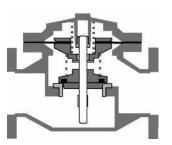
Valve inlet pressure is less than valve outlet pressure. The lift check (lower spool assembly) drops immediately to prevent reverse flow. The valve is closed and flow stops.
