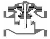
Valve inlet pressure is greater than valve outlet pressure. Pilot system controls valve to open.
