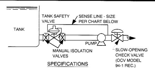
PRESSURE REQ'D TO START VALVE OPEN --- 5 PSID\* PRESSURE REQ'D TO FULL OPEN VALVE ---- 15 PSID\*
