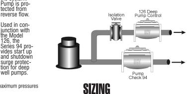
Check valves are normally line size. However for best surge protection the flow velocity should not exceed 15 ft/sec. Definitive sizing information can
