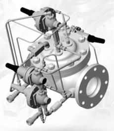
The OCV Model 114-2 is a control valve specifically designed for aircraft refueling service. Known as either a refueling or a hydrant control valve, it is the typical control valve used on pantograph refueling systems. It opens and closes via hydraulic deadman control, while open modulates to control downstream pressure at a predetermined set point, limits flow rate to a predetermined maximum and closes rapidly to prevent undue pressure buildup due to a rapid reduction in demand (HCV).
