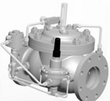
The Model 119-15 is designed to limit the flow of fuel through a filter separator, close fully in the event of high water levels in the filter separator sump and to prevent reverse flow. It operates in conjunction with one of the OCV 800 Series interface float pilots.
