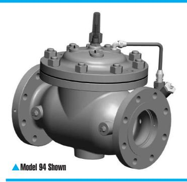
The OCV Series 94 check valve is a simple on-off valve that opens to allow forward flow when inlet pressure exceeds outlet and closes tightly to prevent backflow when outlet pressure exceeds inlet pressure.
