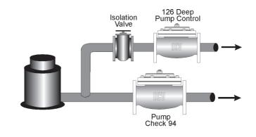
Used in conjunction with the Model 126, the Series 94 provides start up and shutdown surge protection for deep well pumps.
