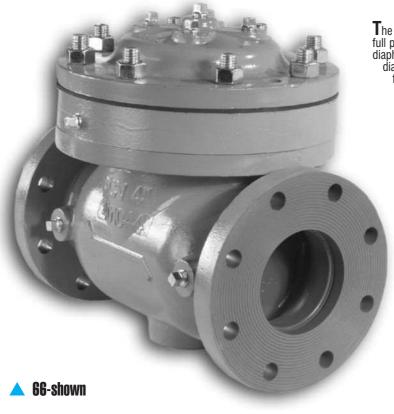
The Basic Control Valve 66 Globe and 66 Angle is a full port engineered valve. Equipped with two diaphragm chambers, sealed from each other by the diaphragm, and isolated from the valve's main flow passage by an intermediate plate. By pressurizing one control chamber while simultaneously venting the other, the valve is positively powered to both open and
