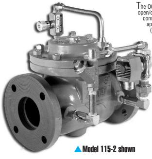
The OCV Series 115 Solenoid Control Valve is designed to provide on/off or open/close control of fluids in response to an electrical signal. The valve consists of the basic OCV model 65 with solenoid-operated pilot. With the appropriate solenoid, the valve may be normally closed (energize to open) or normally open (de-energize to open).
