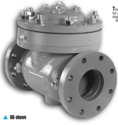
The Basic Control Valve 66 Globe and 66 Angle is a full port engineered valve. Equipped with two diaphragm chambers, sealed from each other by the diaphragm, and isolated from the valve's main flow passage by an intermediate plate. By pressurizing one control chamber while simultaneously venting the other, the valve is positively powered to both open and close.
