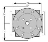
For maximum efficiency, the OCV control valve should be mounted in a piping system so that the valve bonnet (cover) is in the top position. Other positions are acceptable but may not allow the valve to function to its fullest and safest potential. In particular, please consult the factory before installing 8" and larger valves, or any valves with a limit switch, in positions other than described. Space should be taken into consideration when mounting valves and their pilot systems.
