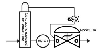
The Model 110 is normally sized to match the meter size; however, in no case should the maximum velocity exceed 20 ft/sec, as shown
