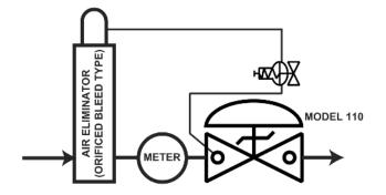
The Model 110 is normally sized to match the meter size; however, in no case should the maximum velocity exceed 20 ft/sec, as shown below.
