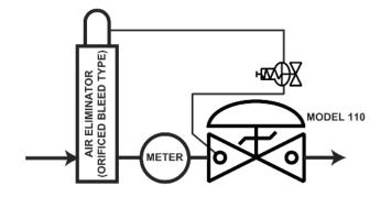
The Model 110 is normally sized to match the meter size; however, in no case should the maximum velocity exceed 6 meters/second, as shown below.
