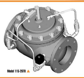
The OCV Model 115-26TR solenoid control valve is designed to open or close in response to an electrical signal. It will also close in the event of a pressure reversal, but will relieve thermal buildup from downstream to upstream. Typical examples include:
