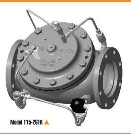
The OCV Model 115-26TR solenoid control valve is designed to open or close in response to an electrical signal. It will also close in the event of a pressure reversal, but will relieve thermal buildup from downstream to upstream.
