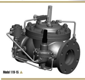
The Model 119-15 has a very specific purpose: to limit the flow of fuel through a filter separator, close fully in the event of high water levels in the filter separator sump and close to prevent reverse flow. To perform this task, the Model 119-15 must operate in conjunction with one of the OCV 800 Series interface float pilots.
