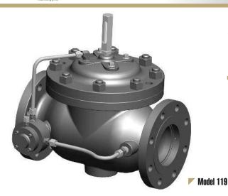
The Model 119 has a very specific purpose: to shut off the flow of fuel through a filter separator in the event of high water levels in the filter separator sump. To perform this task, the Model 119 must operate in conjunction with one of the OCV 800 series interface float pilots.
