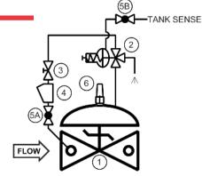
A sense line must be connected within 40 pipe diameters of the tank wall or riser, minimum size of 1/2" 0.D. tubing or 3/8" pipe. In order to prevent accumulation of air, the sense line should slope upwards to the tank. As the 3331 exhausts its diaphragm chamber to diaphragm chamber to atmosphere, the volume
