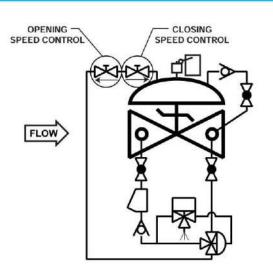
The Model 141-3 Flow Control Valve is shown on OCV Valve Schematics as:
