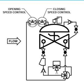
The Model 141-3 Flow Control Valve is shown on OCV Valve Schematics as:
