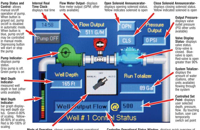
**Mode of Operation**- shows current system operational control mode. Button will display system control by Manual, Off or Automatic. For automatic mode, see F4 functions listed below. Manual mode allows touch screen operation of pump and valve solenoids **Controller Operational Status Window-** displays quick overview of current system status, including normal automatic operations, normal manual operations, and detected errors display (red wording)
