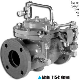
The OCV Series 115 Solenoid Control Valve is designed to provide on/off or open/close control of fluids in response to an electrical signal. The valve consists of the basic OCV model 65 with solenoid-operated pilot. With the appropriate solenoid, the valve may be normally closed (energize to open) or normally open (de-energize to open).
