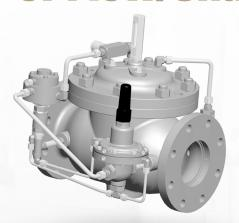
The Model 119-15 is designed to limit the flow of fuel through a filter separator, close fully in the event of high water levels in the filter separator sump and to prevent reverse flow. It operates in conjunction with one of the OCV 800 Series interface float pilots.
