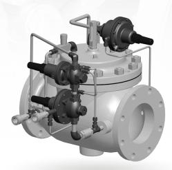
The OCV Model 114-3 is a control valve specifically designed for aircraft refueling service. Known as either a refueling or a hydrant control valve, it is the typical control valve used on pantograph refueling systems. It opens and closes via hydraulic deadman control, modulates to control downstream pressure at a predetermined set point whole open, and closes rapidly to prevent undue pressure buildup due to a rapid reduction in demand (HCV).
