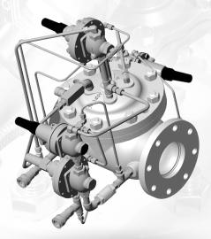
The OCV Model 114-2 is a control valve specifically designed for aircraft refueling service. Known as either a refueling or a hydrant control valve, it is the typical control valve used on pantograph refueling systems. It opens and closes via hydraulic deadman control, while open modulates to control downstream pressure at a predetermined set point, limits flow rate to a predetermined maximum and closes rapidly to prevent undue pressure buildup due to a rapid reduction in demand (HCV).
