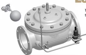
The Model 8104 automatically controls the high level in storage tanks where the float pilot can be mounted inside the tank, such as below ground tanks.
