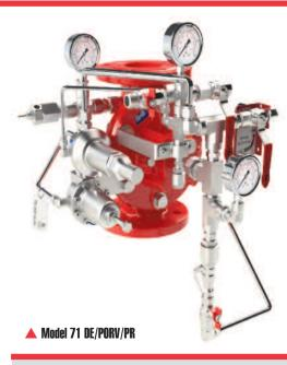
This pneumatically actuated pressure reducing deluge valve is designed for fire protection systems controlled and actuated by an air or nitrogen dry pilot line. The basic control valve type used in this deluge system is a direct sealing elastomeric diaphragm, hydraulically operated control valve engineered specifically for fire protection systems tection systems.
