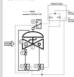
Install the valve at the appropriate location, typically downstream of the preset meter.
