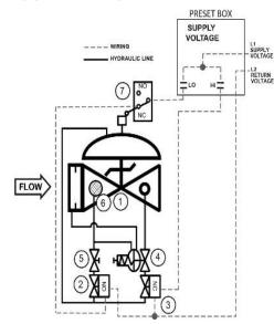
Install the valve at the appropriate location, typically downstream of the preset meter.
