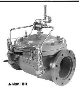
The Model 118-3 operates as a pressure relief valve by opening at a pressure above its set point. In addition, it provides extra protection against surges associated with power failure or other pump failure by opening in "anticipation" of the high pressure wave to follow. By being already open when the high pressure wave hits, any potential surge is harmlessly bypassed to atmosphere. Typical examples include:
