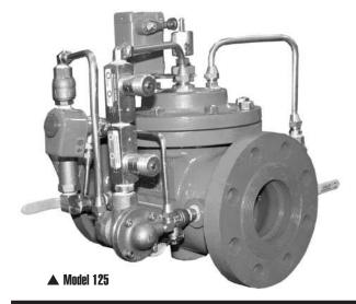
The Model 125, primarily designed for use with centrifugal booster pumps, can also be used on well pumps with relatively shallow lifts where the pump design permits starting against a closed valve.
