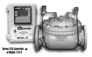
The Model 22S Electronic Pressure Sustaining/Back Pressure Valve provides user pressure control with extreme stability over a wide range of flow. Combining the advantages of simplicity and line pressure operation with the features of electronic control, the valve is able to interface with SCADA systems to provide remote control and programmable variable logic. The electronic feature allows for a wider range of operation, simplifying valve sizing.
