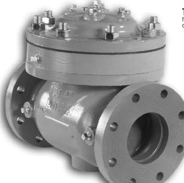
The Basic Control Valve 66 Globe and 66 Angle is a full port engineered valve. Equipped with two diaphragm chambers, sealed from each other by the diaphragm, and isolated from the valve's main flow passage by an intermediate plate. By pressurizing one control chamber while simultaneously venting the other, the valve is positively powered to both open and close.
